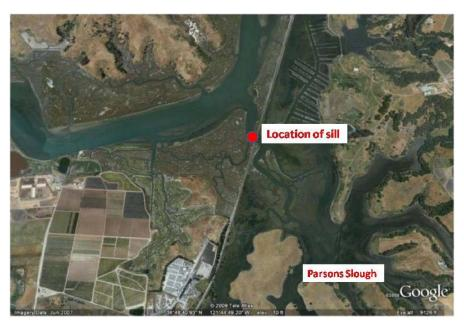
After considering several management options to address the erosion, the Tidal Wetland Project staff and advisors have proposed the construction of a structure, similar to a tidal barrier or an underwater retaining wall, at the entrance to the Parsons Complex. The structure, which is being called a Low Sill, will mute the tidal action in the slough to reduce scour.
