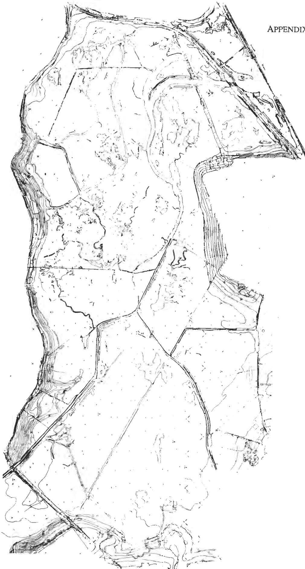
Appendix : Reduction of topographic map of Blohm-Porter Marsh. The large original will be used for construction engineering. Contor interval=1 ft. 1 inch=315 feet.
