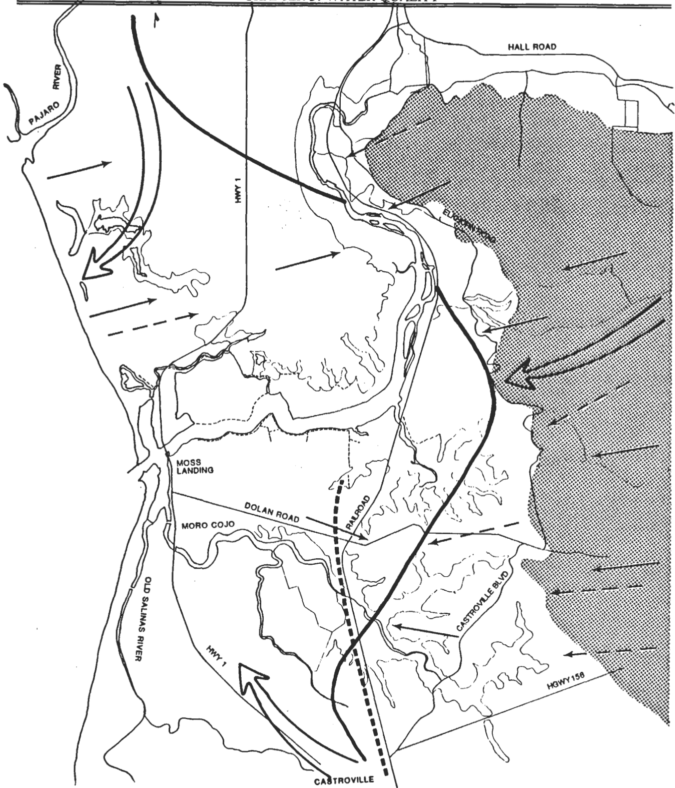
Figure 3-6. Map showing saltwater intrusion and water movement around Elkhorn Slough. Large arrows show groundwater movement in the deep aquifer (Purisima), small dashed arrows show groundwater movement in the lower Aromas, small solid arrows show groundwater movement in the upper Aromas. Solid line shows the axis of the pumping trough in the upper Aromas, dashed line shows the approximate extent of saltwater intrusion in the upper Aromas, and stippled area shows outcrops of the Aromas Sands. Data from Johnson 1983, Leedshill-Herkenhoff 1985, Monterey County Health Department, Monterey County Flood Control District, and personal communications.
